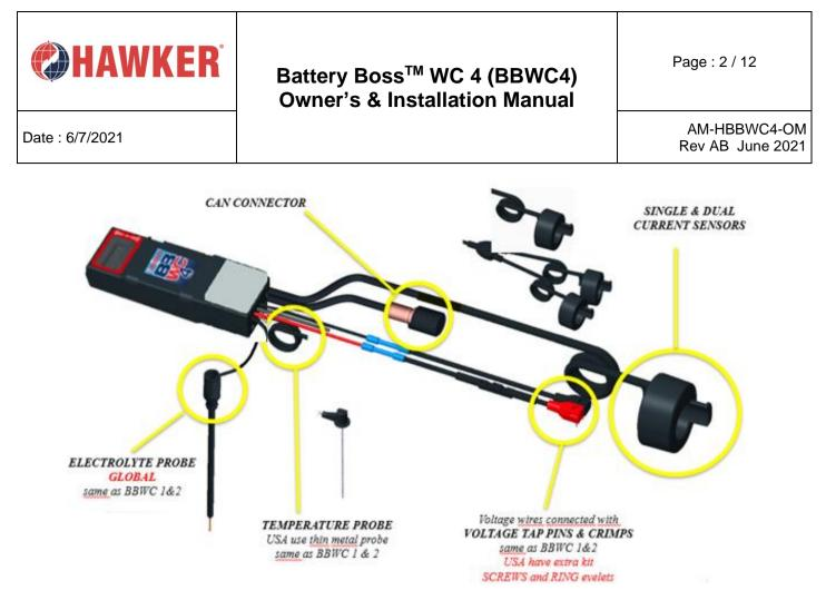
The BBWC4 device can be installed on **24V-80V** batteries.
