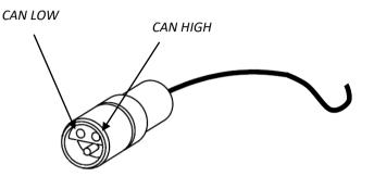
Male connector type not provided = ITT-CANON SURE-SEAL IP68 3-contact receptacle with 2 pins and 1 socket adapted for 0.75-1.5mm<sup>2</sup> wires.
